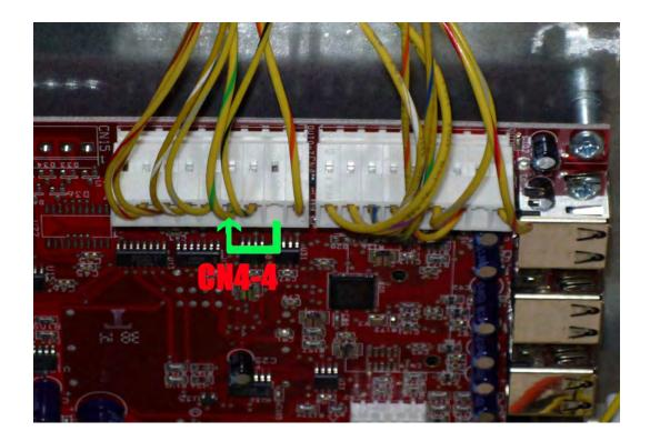
• <u>In the alternative</u> – Add a new wire to the unused Pin 4 of the CN4 housing, and run the new wire to a physical meter or card system ticket input. This will leave the currency meter unchanged and add the new ticket meter output.
