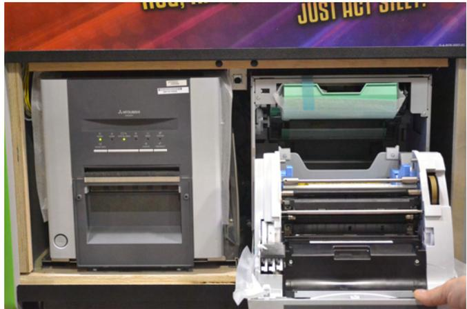
6. Remove all shipping material from inside of the printer.
