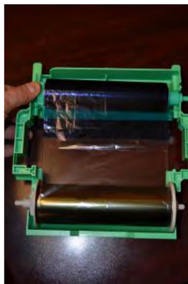
8. The ink film should rotate easily in the support tray.
