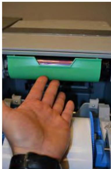
17. Rotate the door upward, until the door locks in the vertical position.
