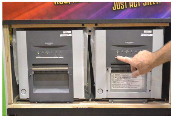
5. The printer will unlock the door and allow the door to be rotated downward.
