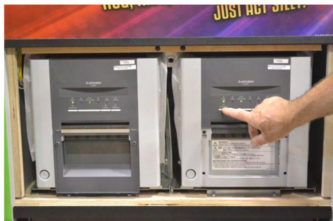
5. The printer will unlock the door and allow the door to be rotated downward. Remove any shipping materials from inside the printer.
