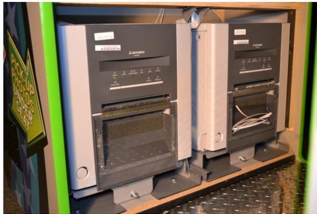
Printers can slide in and out after removing the lower bolt
