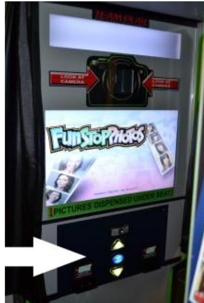
11. Using the keys that were attached to the curtain rod when you received your photo booth, open the control panel / coin door.
