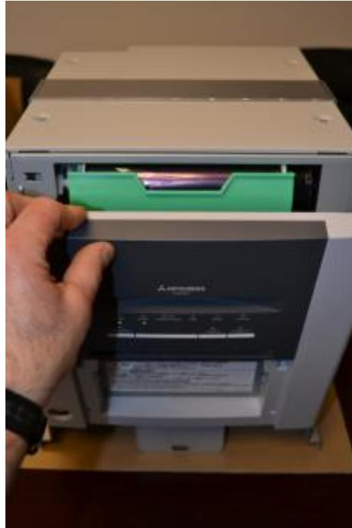
6. Remove all shipping material from inside of the printer.
