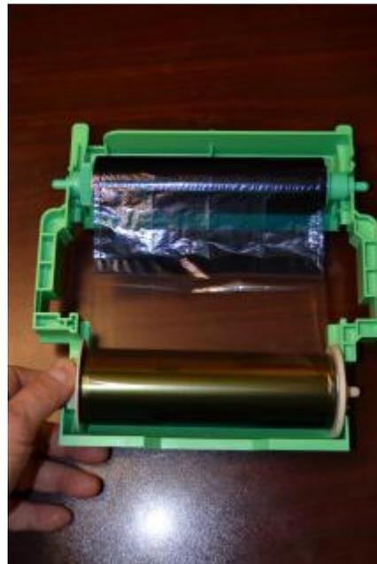
9. Slide the ink film support tray into the top of the printer.
