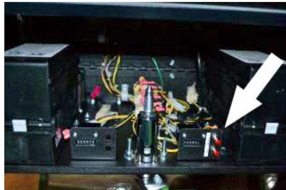
13. The TEST button is the red button on the bottom. Pressing the TEST button will activate the Adjustments and Audits menu on your screen.
