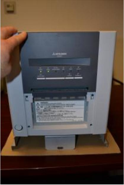
13. After the door is locked into place, the printer will automatically feed four sheets of paper to test whether the paper is installed properly.
