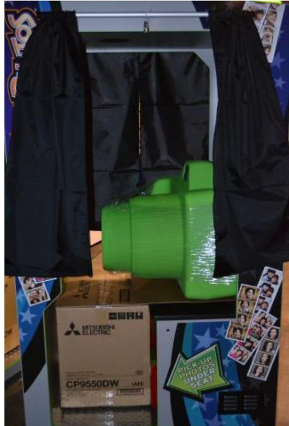
2. Lift the cabinet off of the pallet and remove the shrink wrap. Be careful not to cut into the photo booth, as you will cut the artwork decals.
