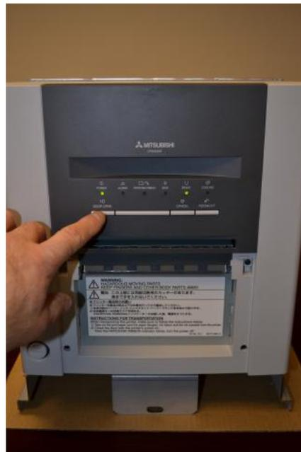
5. The printer will unlock the door and allow the door to be rotated downward.
