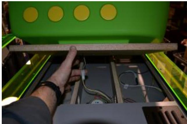
9. Secure the camera and access panel to the top of the cabinet using the two bolts that were removed earlier.
