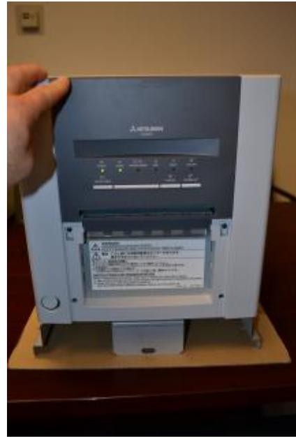
18. The “READY” light will turn green on the printer once the ink film and paper have been loaded properly.
