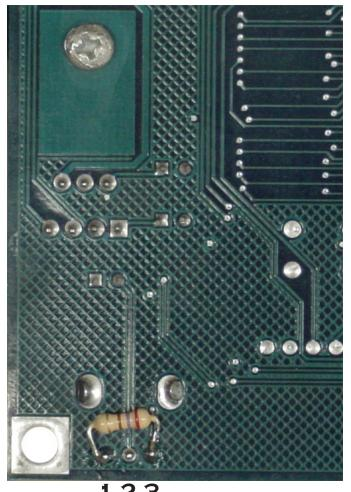
SIMPLY SOLDER A 270 OHM RESISTOR BETWEEN PINS 1 AND 3 OF THE VOLUME POTENTIOMETER ON THE BACK OF THE PCB. THE COLOR BANDS ON A 270 OHM RESISTOR ARE:
